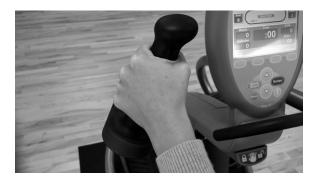
2. To lock the arms and pedals, push the StrideLock button. Verify that the lock is engaged by pushing or pulling the upper arm grip.
