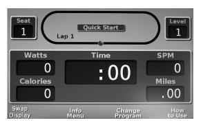
This program automatically starts just by moving the arm handles or foot pedals. It also bypasses entering goal information. The user can manually change the workload as desired by using the up and down arrow buttons.
