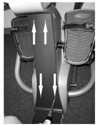
3. Remove 2 screws from right upper cover and remove cover from frame.
