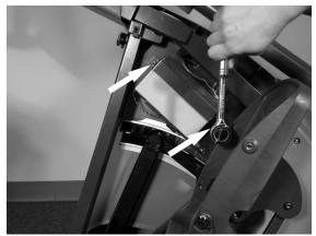
5. Remove the battery cables.
